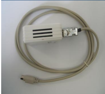
SM_T_H_COM - Optional Temperature and Humidity Sensor for direct connection to COM 2 port of a CS121
